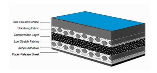
Available in a range of thicknesses; 0.90mm 0.95mm 1.00mm 1.05mm
