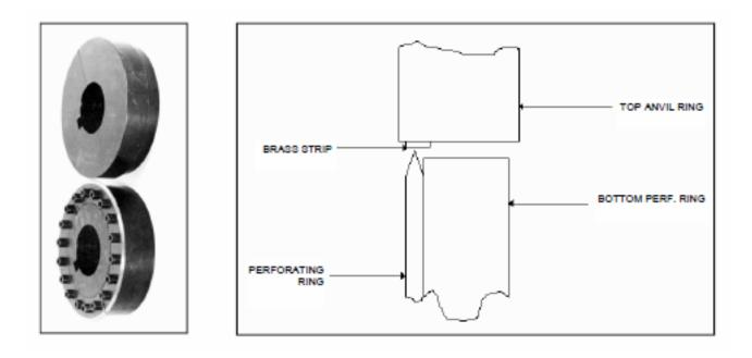
The lower ring is for mounting the split perforating rings which are made in two halves and come in any variation of cut and tie to suit all requirements, including micro perforating.
